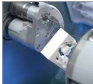
MILLING AND GRINDING of restorations and pin models with the inLab MC XL.
