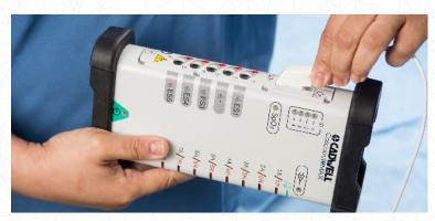
SpO<sub>2</sub> Measure pulse oximetry and heart rate from up to four limbs.
