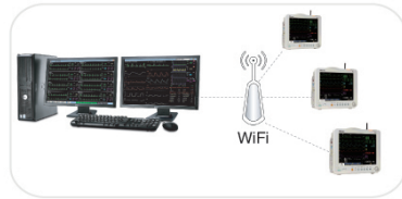
Wire / wireless network solution Bi-directional communications with central monitor station by wire / wireless network Nurse Call
