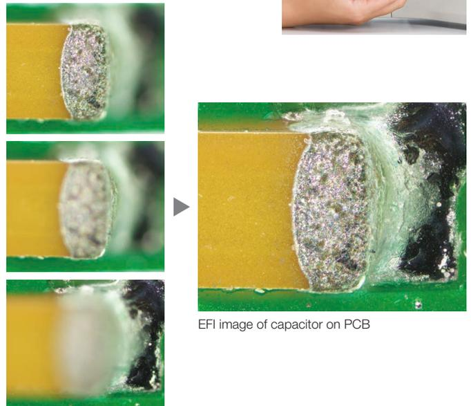
EFI image of capacitor on PCB
